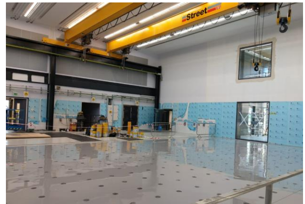
22. Structures lab with 2no. 10t gantry cranes and strong floor.
